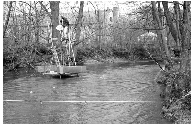
Figure 1. Application of PTV for field studies in the Wesenitz River, Germany.
