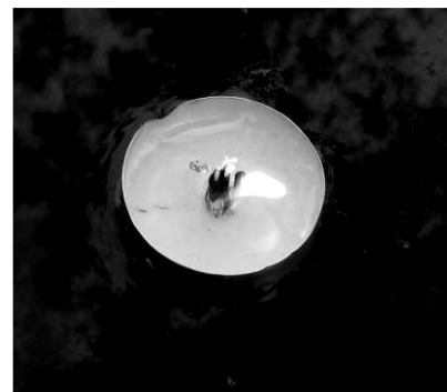
Figure 3. Tea candle as a tracer particle for free surface field PTV or PIV.
